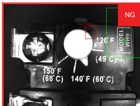
The dial on a thermostat is checked to confirm that it is in the correct position, which helps to ensure proper installation.
