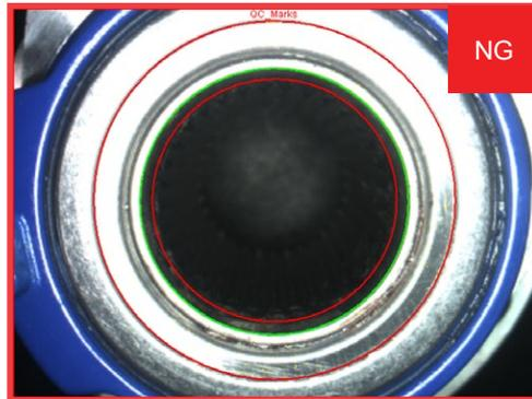
A wheel hub bearing is checked for the presence of quality control (QC) marks before moving to the next stage of assembly. The absence of the QC marks indicates that the hub bearing has not yet been inspected.
