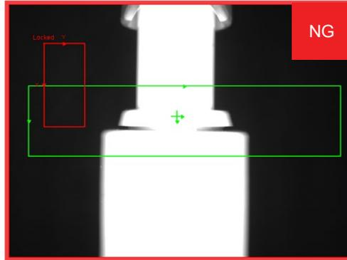
A lotion bottle is checked to confirm that the pump dispenser is in the locked position before the bottle is packed into a carton.
