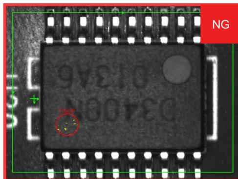
The presence of a fiducial is used to verify that an integrated circuit has been soldered onto the PCB in the correct orientation.
