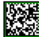
Quiet zone violation
